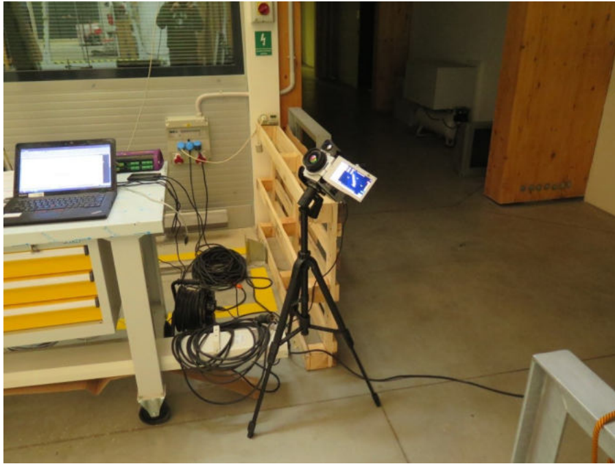
Figure 4-6 Thermal imaging camera used for control of panel's surface temperature
