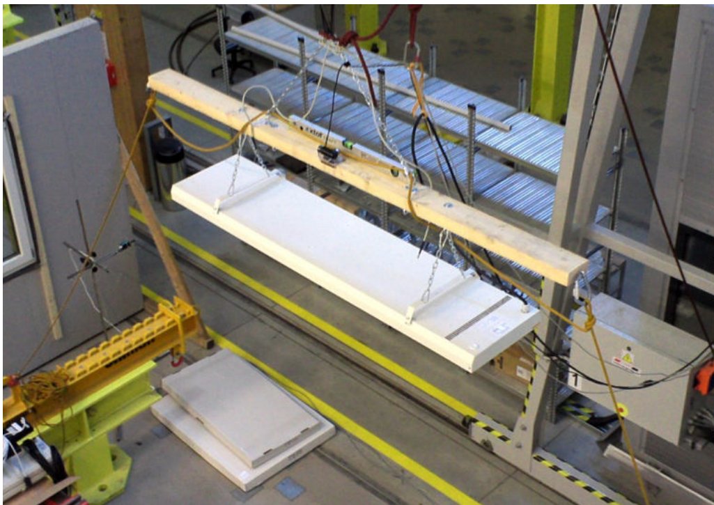
Figure 4-3 Radiant panel Ecosun S+ 30 suspended on auxiliary structure during stabilizing period (rear view)
